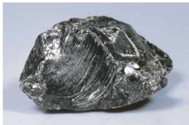
Figure 3-10 Quartz typically fractures along smoothly curved surfaces, called conchoidal fractures. This sample is smoky quartz. (Breck P. Kent)
